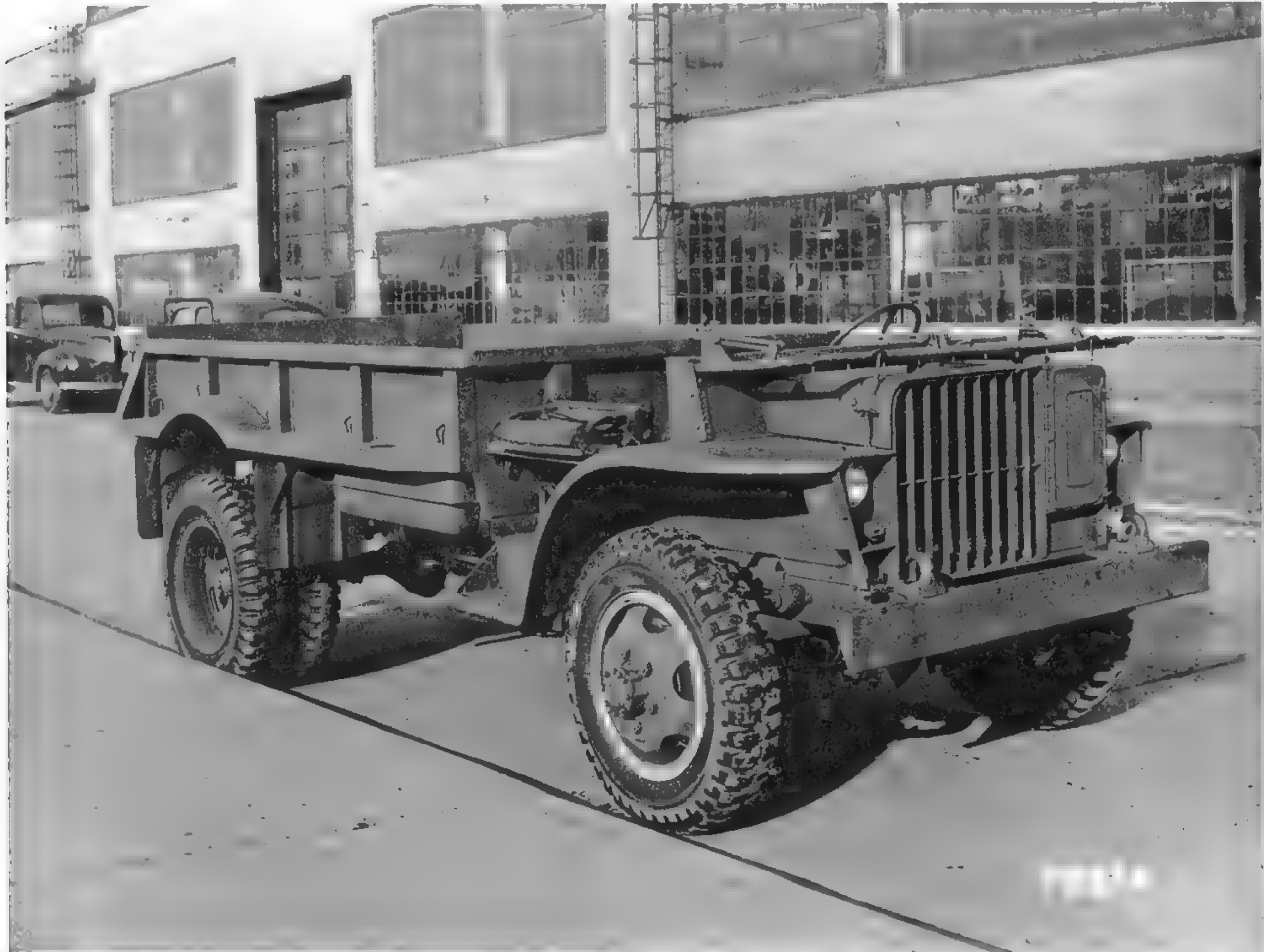
This is the very first Ford GTB. It differs from the production model in that it lacks a blackout-driving lamp, and it has no windshield wiper motors. These trucks' ancestry in the low-silhouette program is apparent in this view. The passenger's seat back has been folded over. (Photo courtesy of the Bryce Sunderlin collection)
